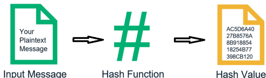
Slika 3. Kriptografski hash u akciji. Izvor: https://sectigostore.com/blog/hash-function-in-cryptography-how-does-it-work/
